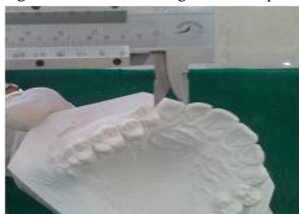
Figure 2: maximum mesiodistal dimension of maxillary right canine using vernier calipers.
